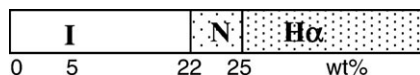
Scheme 2 Phase diagram of aqueous solutions of CTAB (25 °C): I-isotropic, N-nematic and H \alpha -hexagonal liquid crystalline phases.
